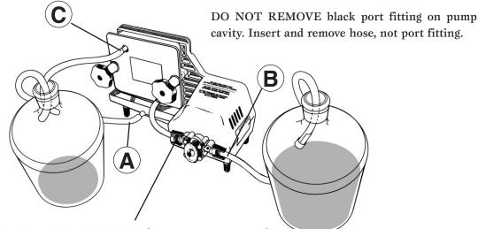
TO REMOVE WHITE HOSE CLIP: (Output port on pump)
